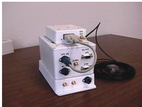
Figure 3. Packaged GPS-disciplined oscillator for the sounder.
